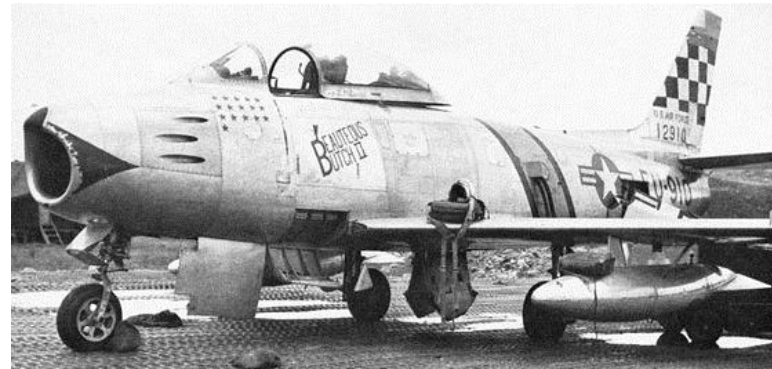
The famous “Beauteous Butch II”, personal aircraft of the top scoring ace in Korea - Capt. Joseph McConnell. Note that the blue nose scallop is peeling badly due to sustained high Mach numbers. The tall stripe is yellow; the aircraft name is red. (NAA)
