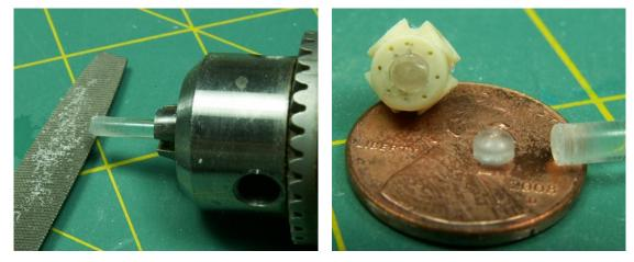
The "PE" wheel well parts were not made right, so I scratch-built everything in.
